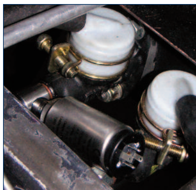
1500 Series pressure sensor being used to test hydraulic brake performance.
